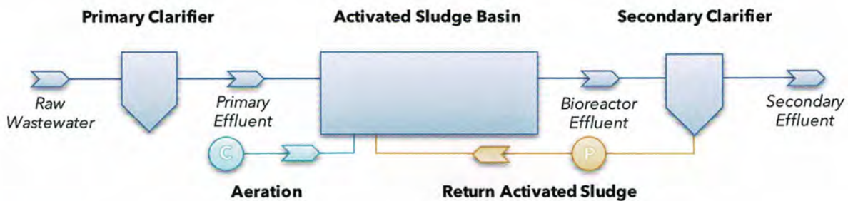
Flow Chart of Conventional Wastewater Treatment Process
